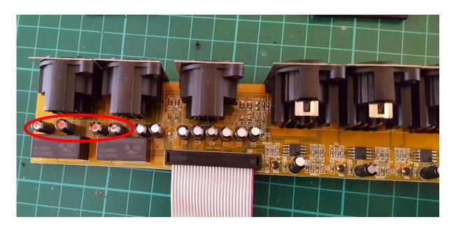
Locate and remove capacitors C26, C27, C41, C42
