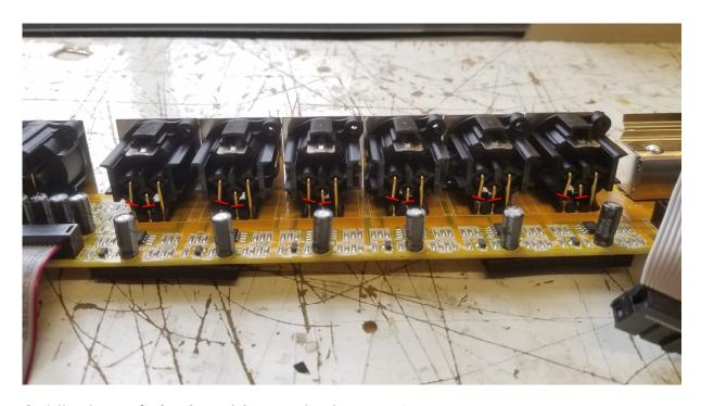
Cut the legs of pins 2 and 3 on output XLRs 1-6.
